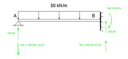
$$R_A = R_D = 150 - 24,35 = 125,65 \text{ kN}$$
